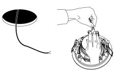
**5** Lift one clamp of the loudspeaker and insert it into the hole paying attention to not hurting the hands.
