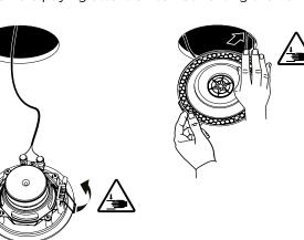
Lift the other clamp and insert in into the hole in order to set the loudspeaker in its final position.
